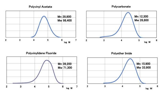
Figure 5. Absolute molecular weight distribution of polymers in KJCMPA®-100
