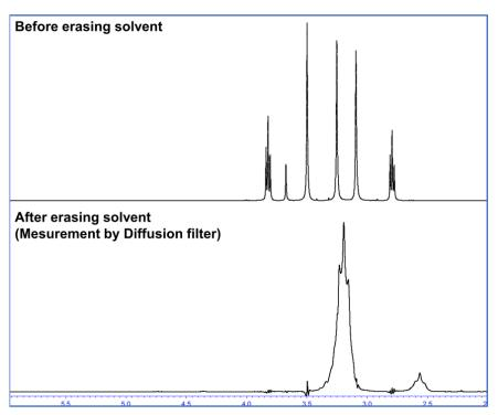
Figure 6. Comparison of NMR spectra with or without diffusion filter
