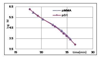
Figure 4. pMMA, pSt calibration curve in KJCMPA<sup>®</sup>-100
