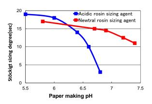
Figure 13. Comparison of the performance of acid and neural rosin sizing agent at different pH Paper-making conditions:
