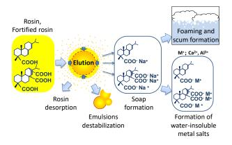
Figure 11. Problems caused by "elution" of rosin
