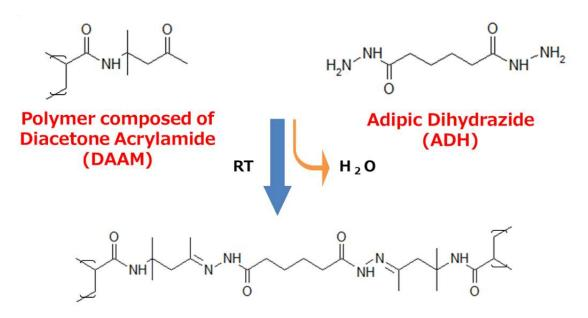
Figure 2. Reaction of polymer composed of diacetone acrylamide with adipic dihydrazide
