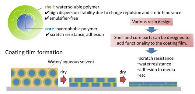
Figure 1. Core-shell polymer emulsions and coating film formation
